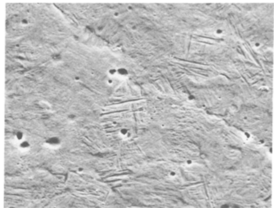
Figure 14 SEM micrograph of the interface joint showing regions where fusion has taken place and regions where it has not. Specimen heavily etched ( \times 1165 ).
